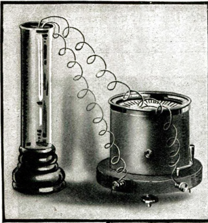
Above: A Coil of Special Wire Is in Circuit With a Current Meter; the Coil Is Immersed in the Liquid Air. The Current Increases As the Temperature Is Lowered, and the Reading Gives the Temperature.
