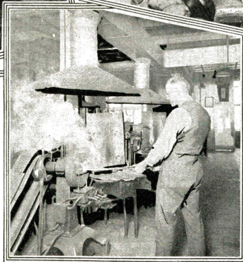
Above:—After Tungsten Has Been Swaged Down to Heavy Wire, the Drawing Process Begins. Here It Is Being Drawn Thru a Gas Flame and Then Thru a Die Reducing It From 0.030 to 0.014 Inches. It Is Tough and Thoroughly Ductile by This Time, But Is Far Too Large for Lamp Filaments.
