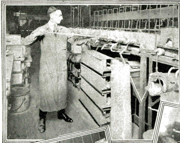
Below We See the Last Process in Using Tungsten in Lamps—Winding the Fine, Tangle Wire on the Lamp Mount by Hand.
