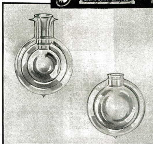
Dewar Glass Flasks With Double and Triple Walls For Holding Liquid Air.
