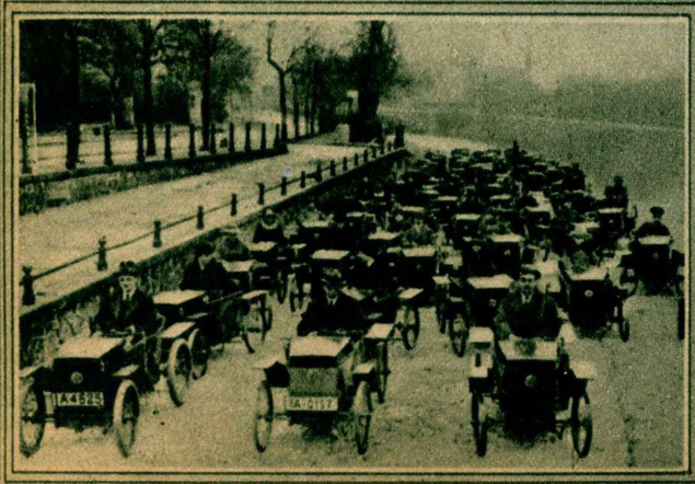
Below—Latest Electric Motor Car Being Built by the Thousand in Germany. It is Run by a Dry Battery Renewable Every 4 Hours. Speed 17 1/2 Miles Per Hour.
