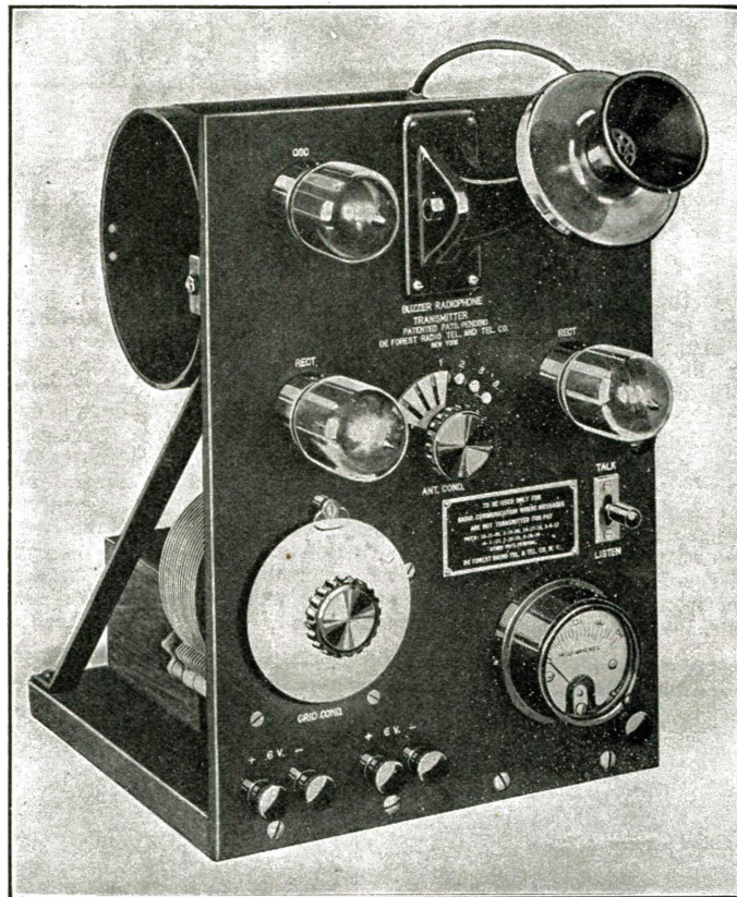
The Very Latest in Radiophone Sets. It Talks on Two Six-Volt Storage Batteries—No "B" Battery Required. Just the Thing for Motorboats, Camping Parties, Motorcycle, Automobile or Airplane.
