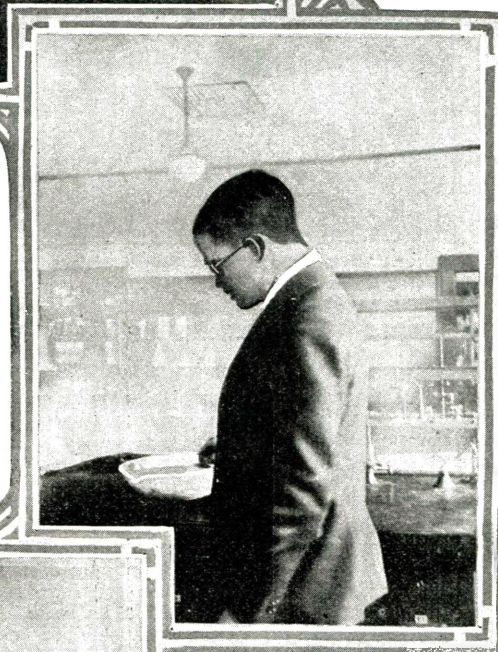
Preparing Blue Print Paper By Lightly Drawing a Piece Over the Sensitizing Solution.
