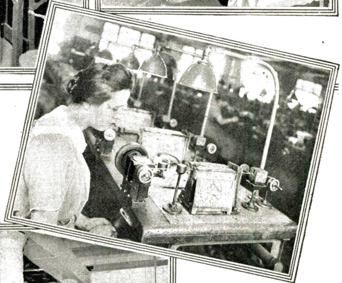
Above:—Drawing Tungsten Down to Finest Proportions, About Four Ten-Thousandths of an Inch or One-Sixteenth of the Size of Fine Human Hair, and Which Cannot Be Seen Except Against a Background If Exactly the Right Color. It Is Used as Filament in the Smallest "Bug" Lamps. The Thread of Tungsten Unwinds From the Spool at Extreme Right, Passes Thru Small Box of Lubricant, Then Thru Gas Furnace Which Has a Diamond Die at Its End Nearest the Operator. The Wire Then Winds on a Receiving Spool and Is Ready to Be Put Into the Tiniest Lamps.
